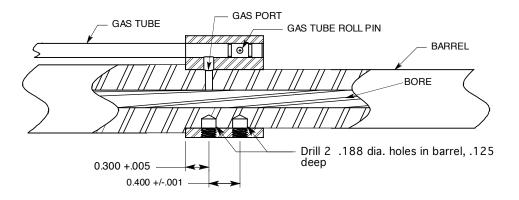
RECOMENDED: Apply a small amount of #262 (red) Loctite to the set screws and around the gas port.
