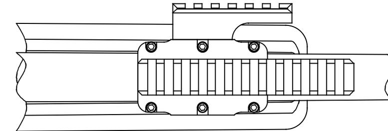
Barrel diameter 1.15" at rear of mount
